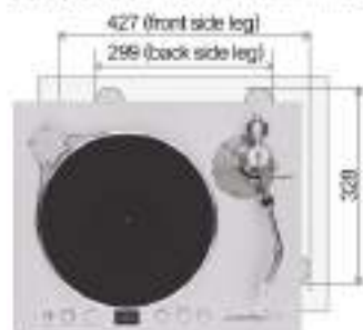
Insulator position / dimensions (all dimensions are in millimeters)
