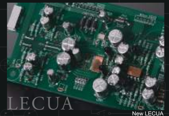
ODNF Power amplifier block of parallel module ODNF version 4.0
