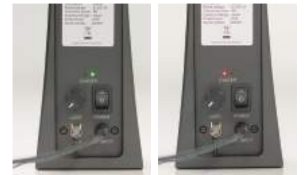
○If the lamp is green, it is operating normally ×If the lamp is red, there is a problem with the operation
