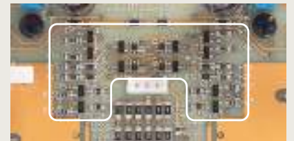
2-parallel circuit layout of MCS+ principle
