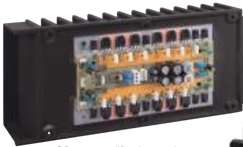
⑮ Power amplification section
