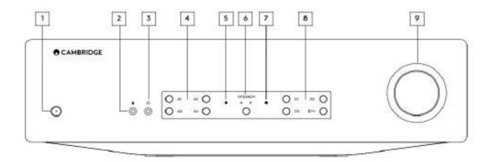
**1. Standby/On** - Switches the unit between Standby mode (indicated by dim power LED) and On (indicated by bright power LED). Standby mode is a low power mode (0.5 Watts). The unit should be left in Standby mode when not in use.
