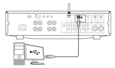
**Important Note:** Always turn the volume to minimum, switch to another input or turn the CXA off before plugging/unplugging cables to the USB input or whilst booting up/shutting down your PC/Mac.
