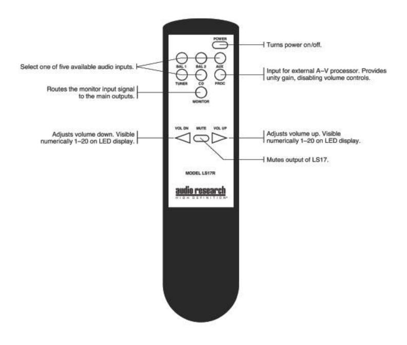
NOTE: All LS17 SE functions are available on the LS17R hand held remote controller. All functions are indicated on the front panel as they are selected. See 'Description of Controls' in this manual for more information.
