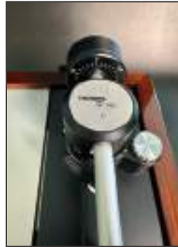
Fig. 8 Bearing block, installed counterweight with scale for the bearing force and anti-skating adjustment.
