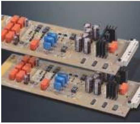
Phono equalizer with separate mono construction for left and right channel
